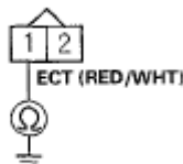
ECT SENSOR 1 2P CONNECTOR
